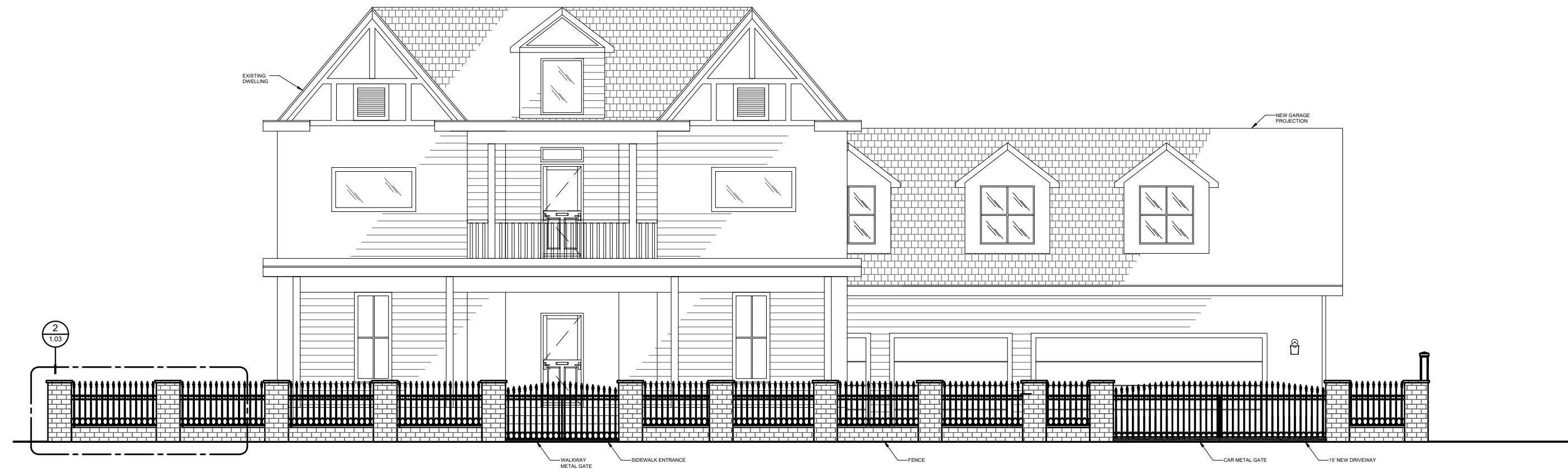
BRICK & METAL FENCE EXTERIOR ELEVATION D SCALE: 3/32" = 1'-0"
